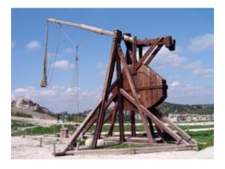
which is allowed to rotate around a fixed axis. The shorter end of the pole is attached to a very heavy weight to counterbalance the projectile. When the weight is released at the short end, the pole rotates, flinging the stone at high speed upward and toward the enemy.
